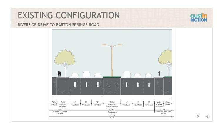
This is the typical section for the existing configuration of South Lamar between Riverside Drive and Barton Springs Road.
